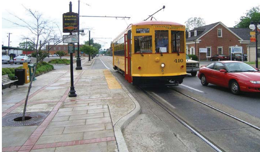
Many newly constructed streetcar lines utilize “bulb out” platforms at stops. This arrangement places the streetcar track in a traffic lane while preserving on-street parking. In this example from Little Rock Arkansas, the “stop” is configured in a no-frills fashion, with no waiting shelter.
