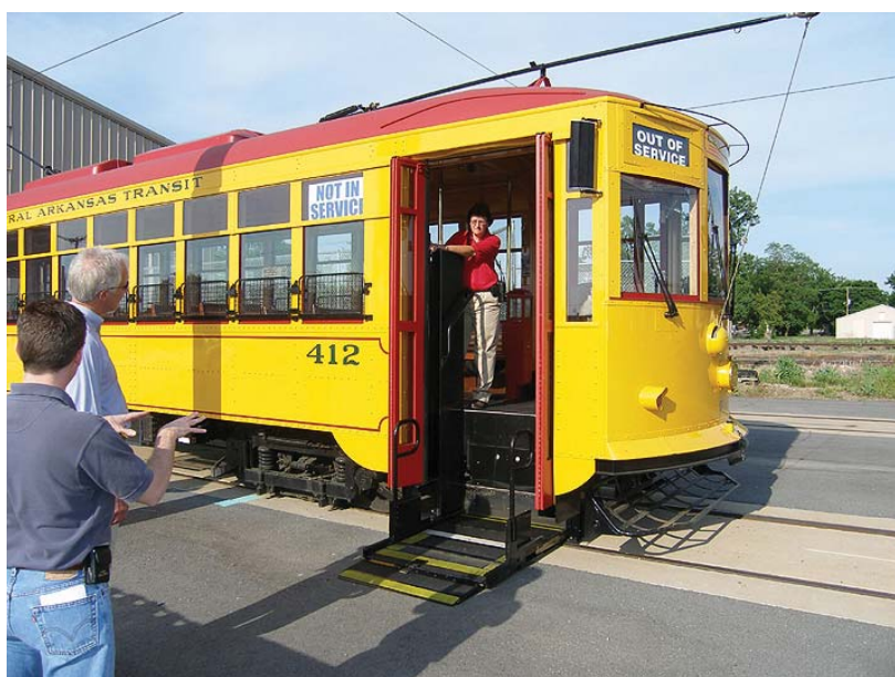
Example of an onboard wheelchair lift. When not in use, lift forms stairwell for normal walking entry into car.
