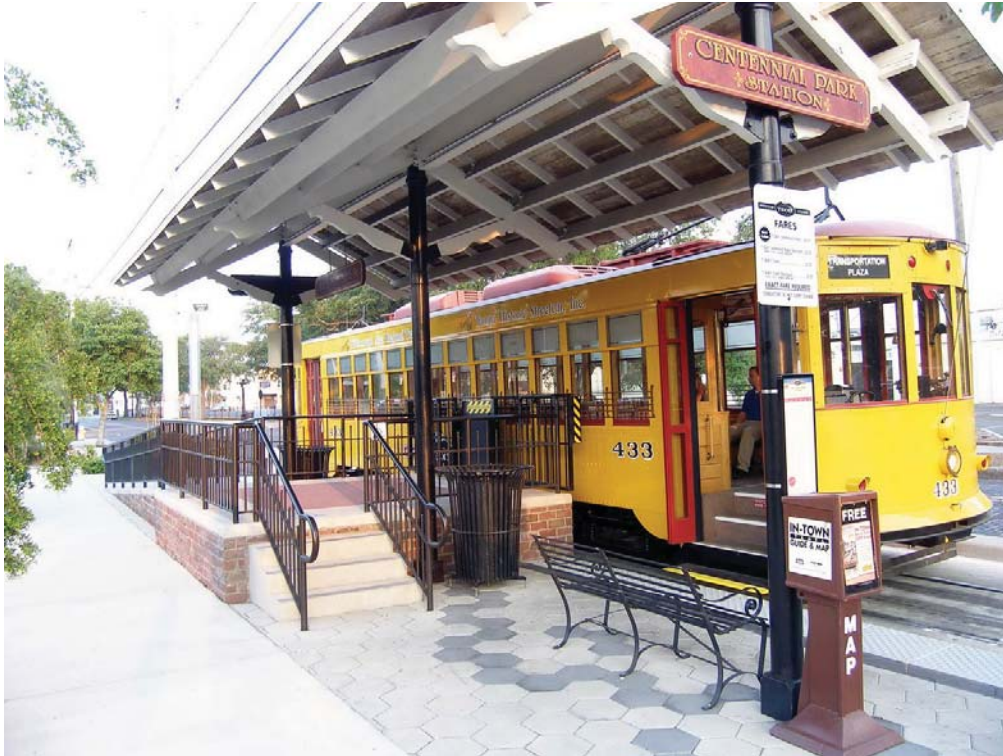
Several of the station on the Tampa streetcar system have a “heritage” look. This station platform shares space on the sidewalk and incorporates a high-block platform and ramp for on-demand ADA access. Normally the streetcar simply stops at the curb.
