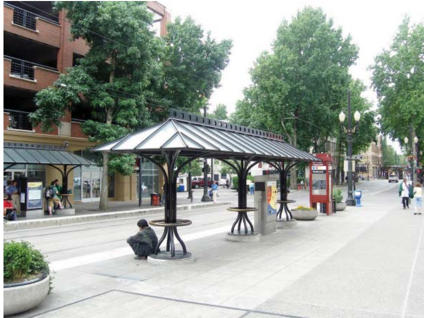
A more elaborate waiting shelter on the downtown light rail alignment in Portland, Oregon. This shelter incorporates a “heritage” theme that blends well with the adjacent historic district. The shelter is relatively large based on the passenger volumes associated with the multi-car light rail trains.
