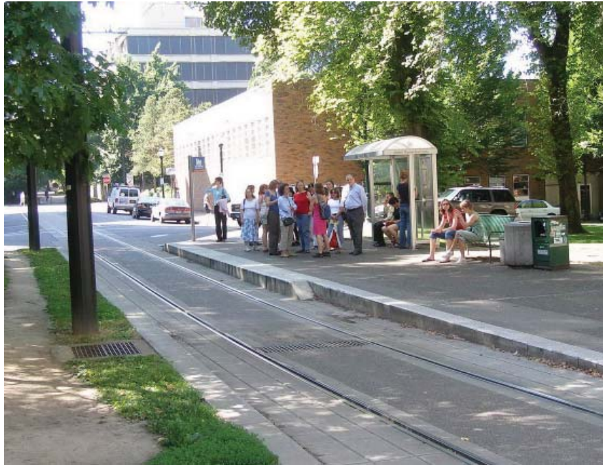
Typical streetcar stop, Portland, Oregon. The stop has a shelter, an additional bench, trash can, basic signage, and a real-time arrival sign inside the shelter. Stops on streetcar lines are typically not elaborate- the streetcar tracks make it easy for system users to locate the streetcar route, and with stops closely spaced, they're easy to find.
