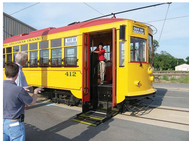
Vehicle-borne wheelchair lift applied to streetcar
