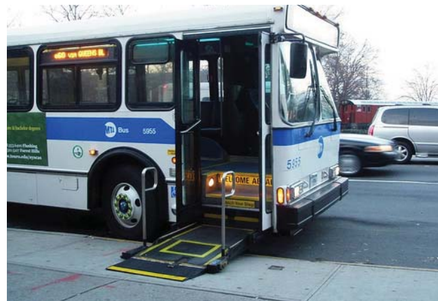
Vehicle-borne wheelchair lift applied to bus
