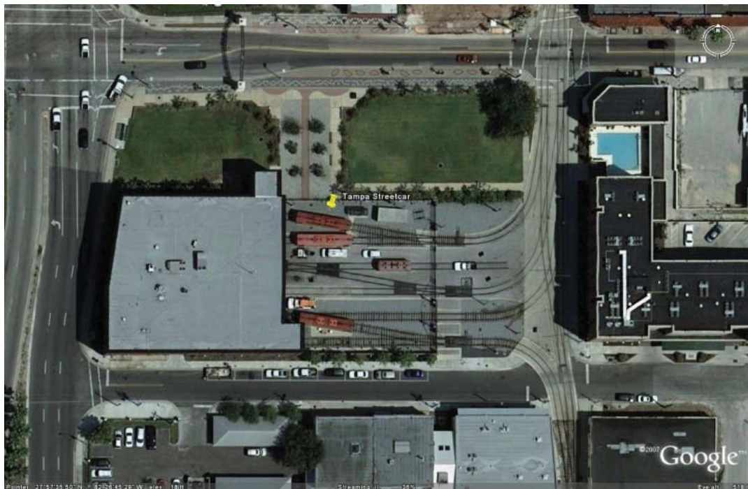
An example of how a streetcar shop can be fit into an urban environment, Tampa, Florida. Note that the entire yard and related access trackage is paved, allowing vehicles to easily move over the streetcar trackage. The yard area immediately in front of the building is also fenced. Employee parking is accommodated with both on-street parking and parking within the yard area. The facility has a 17,100 s.f. footprint, almost identical in overall size to the proposed Red Car facility
