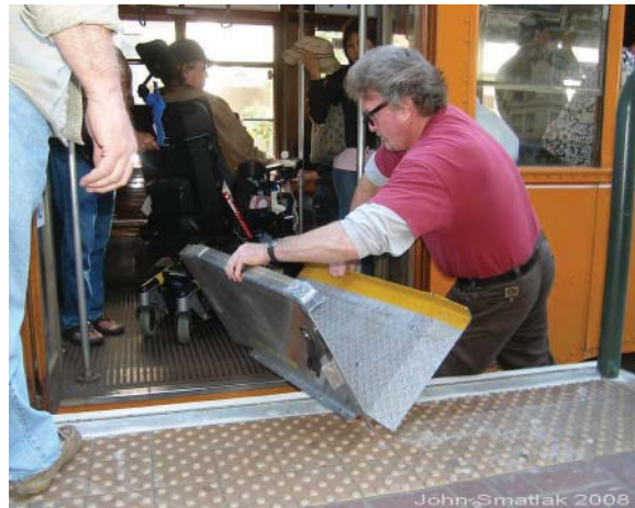
Operator deploying portable bridge plate to span gap at high-block platform
