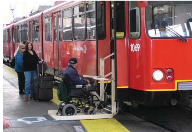
Vehicle-borne wheelchair lift on San Diego Trolley light rail system
