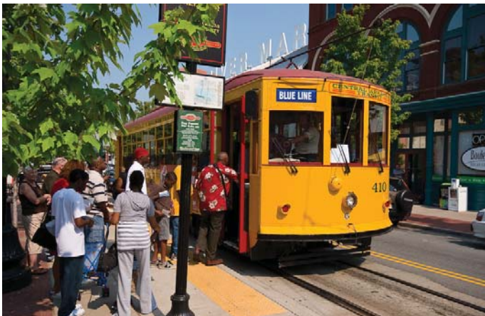
Boarding a streetcar from a sidewalk platform in Little Rock Arkansas. ADA access is provided by an on-board wheelchair lift which deploys on demand.
